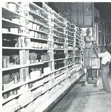
(7) Stacking kiln for firing.
