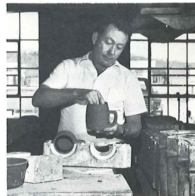
(2) Removing piece from mold.
